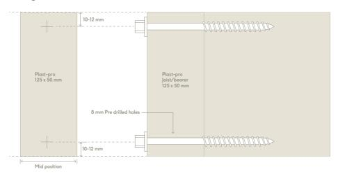
NOTE: Screw fixing method using Durafix hex head screws is for braces or noggins. If a joist is to be fixed then the use of truss clips with screws is recommended
